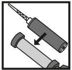
4. Place the Sikadur® Injection Resin cartridge into the application gun ready for use
