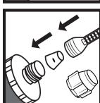
2. Fit the cartridge outlet plug into the cartridge then place injection resin mixer nozzle onto the cartridge
