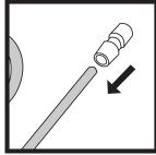
6. Fit push fit connector onto the hose. Pump gun until both resin parts are extruded as one mixed consistent colour. Do not use unmixed material. Place connector over an injection port and start the injection application.
