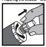
1. Unscrew and remove the cap
